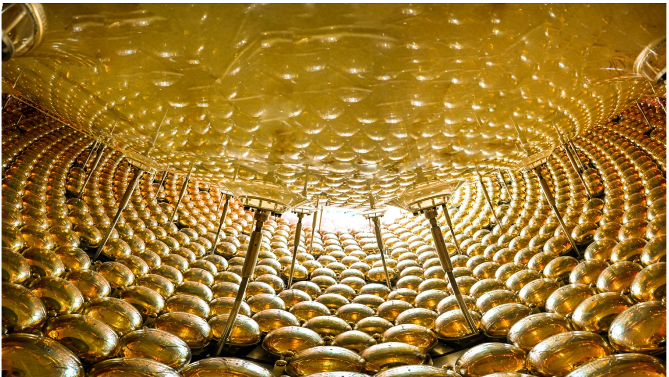
Fig.7 : JUNO central acrylic sphere with its support bars, surrounded by the large photomultipliers tubes (PMTs).
