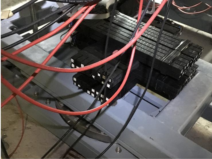
Figure 4.1: The hodoscopes were placed in a Jenga-like pile under the demonstrator such that tracking could be performed in both directions.
