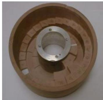
Figure I-11 – Picture of a range modulator wheel with three range modulation tracks (IBA) [47].
