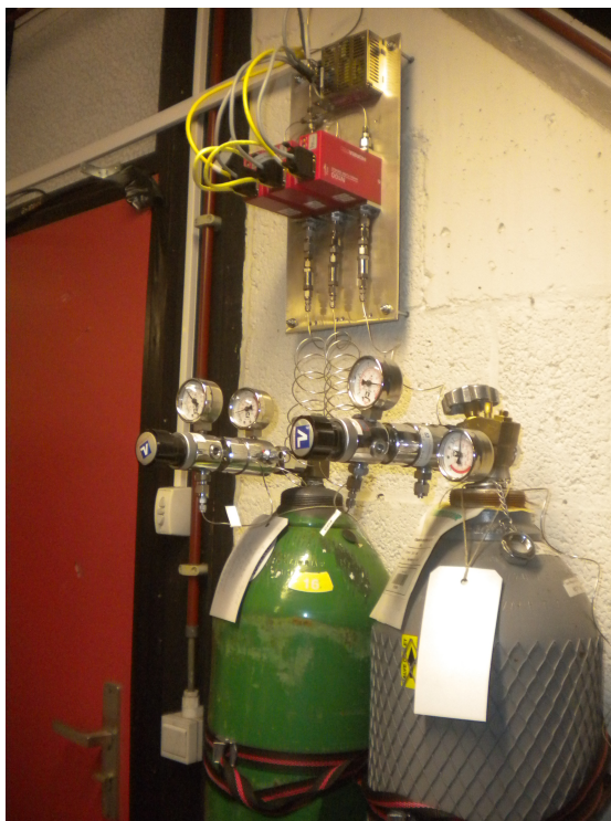
FIGURE 5.10: The two gas bottles and the HORIBA flow meters remotely monitored via Ethernet.
