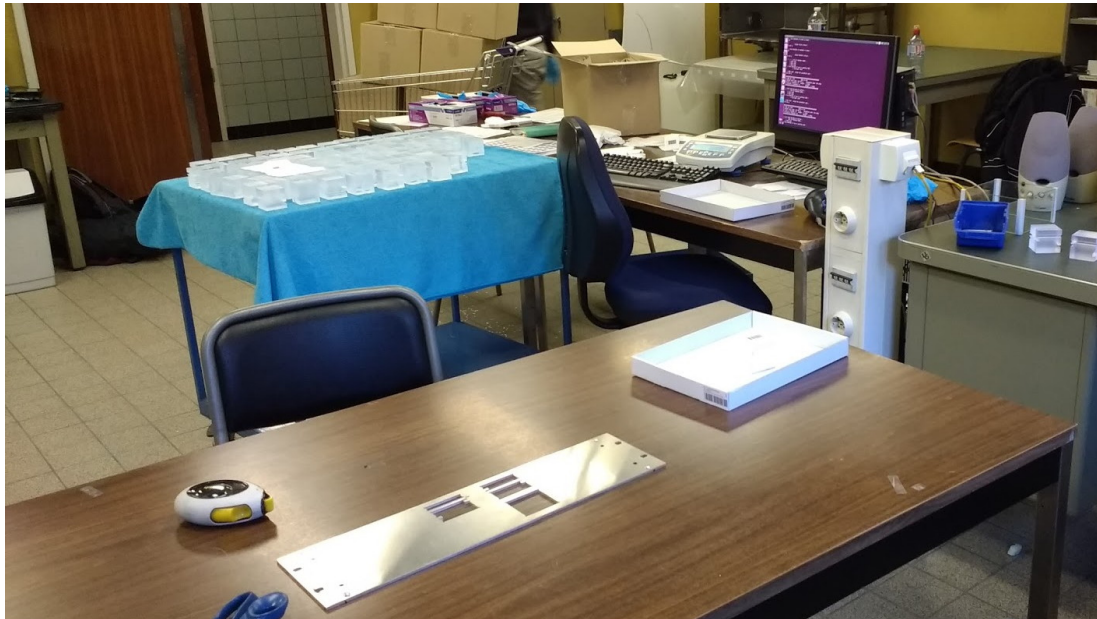
Figure 2.9: Cube wrapping setup in Ghent, Belgium. In the top right of the picture is the computer with connection to the database. Attached to the computer is a scale to weigh the bare cube and the bare lithium screens and a barcode reader to keep track of the cube number, PVT batch number and lithium screen batch number. When all these values are introduced in the database, the parts are brought to the table in the front of the picture where the cube is wrapped. The cube is oriented using the metal tool on the table, placed in the Tyvek wrapper with the aligned neutron screens and closed with tape. The metal tool also serves as a check on the cube size, cubes that are too large to fit in the extrusions are rejected. The wrapped cube, i.e. an assembled detection cell, is then returned to the first table so it can be weighed again and stored until it is placed in a frame.
