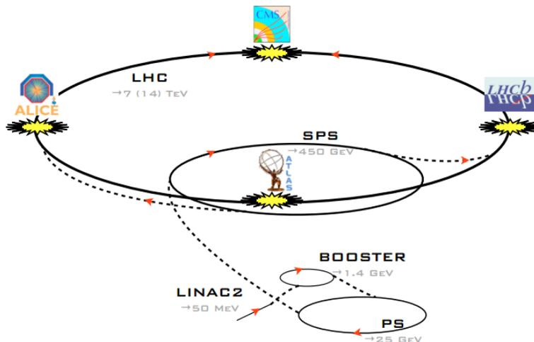
Figure 1.4: Sketch of the Large Hadron Collider, its preaccelerators and the four main experiments (CMS, ATLAS, LHCb and ALICE) at the interaction points (not to scale) [27].
