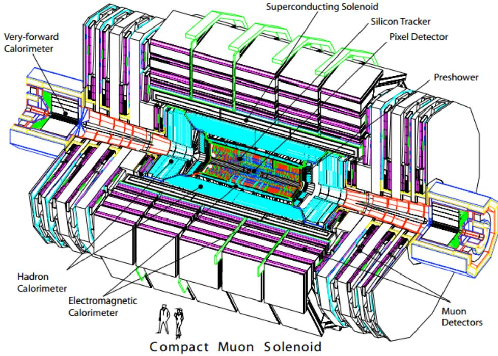
Figure 1.5: Overview of the CMS detector and its different subdetectors [29].
