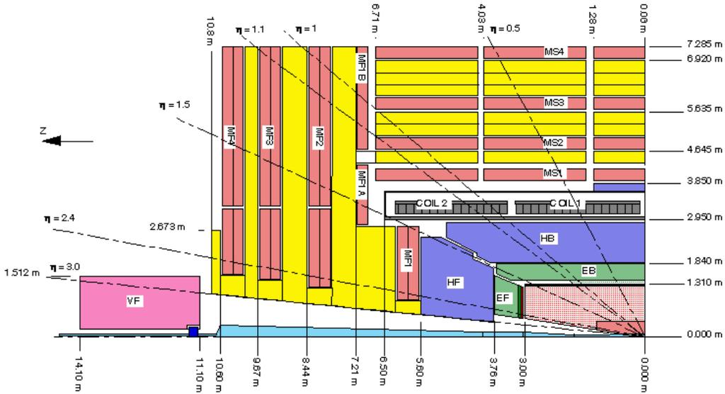
Figure 1.6: Schematic side view of the different CMS subdetectors and corresponding  $\eta$  coverage. From inside-out: The inner tracker (red), the ECAL (green), the HCAL (blue), the solenoid magnet (gray) and the muon chambers (pink) interleaved by return yokes (yellow) [30].
