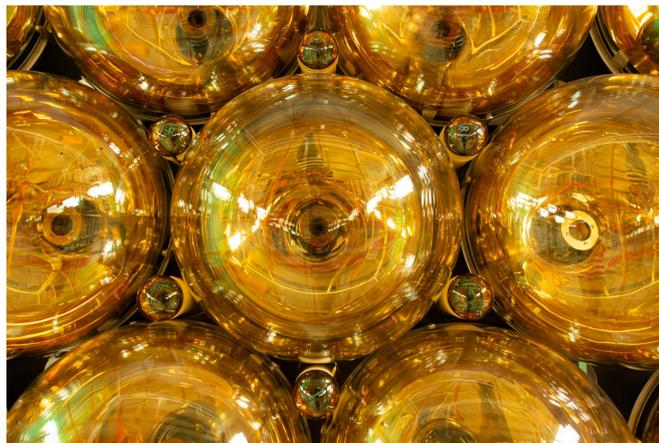
FIGURE 2.2: LPMT and SPMT positioning. The SPMTs are positioned in the interstices of the LPMTs. Taken from [64].
