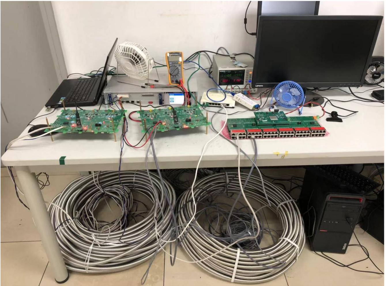
FIGURE 5.30: Setup of BEC-GCU synchronization test. Two GCUs (on the left) are connected to the BEC-V4. The tests were performed in IHEP, and the picture is taken from [190].
