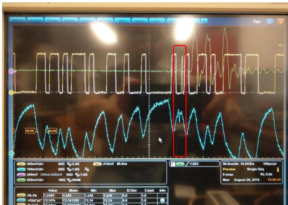
FIGURE 5.34: The errors are captured during a long-term test. In order to have a clear view, we have moved the delayed version of the original data to overlap with the received data after the equalizer.
