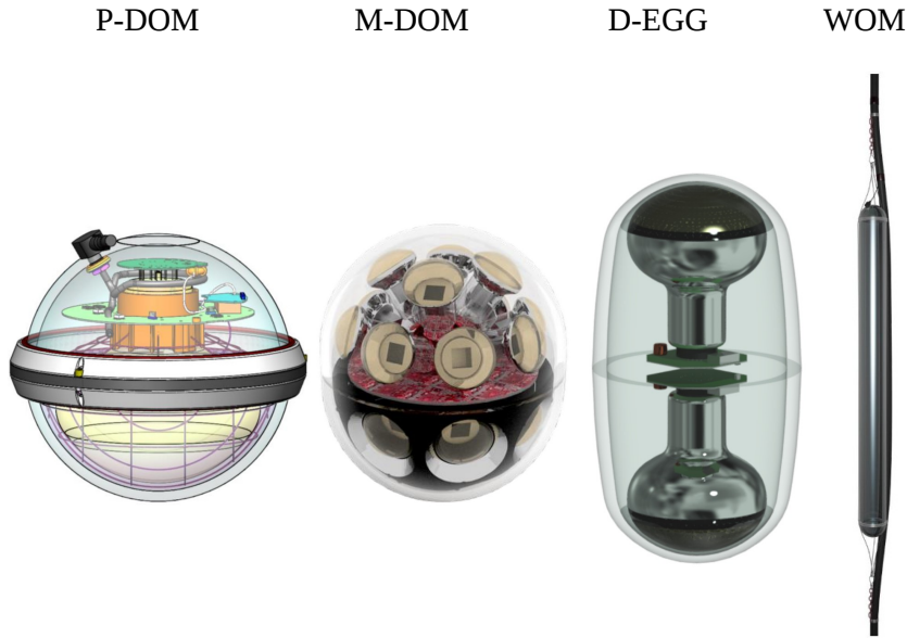
Figure 10: Proposed DOMs which are to be used for the high-energy InIce extension [44].
