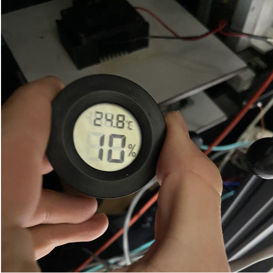
(a) Relative humidity measurement inside the light-isolated cabinet.
