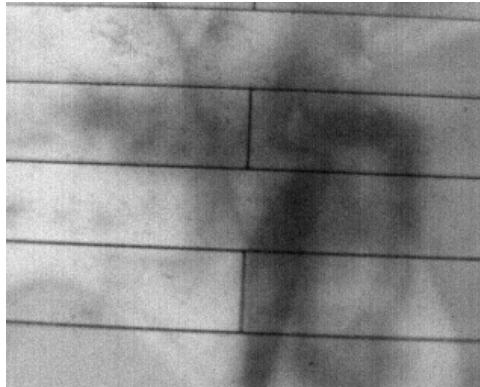
Figure 3.12: EL image of the scratched solar cell on the metallic backside, forward biased at 70mA, acquired with a 10mm spacer.
