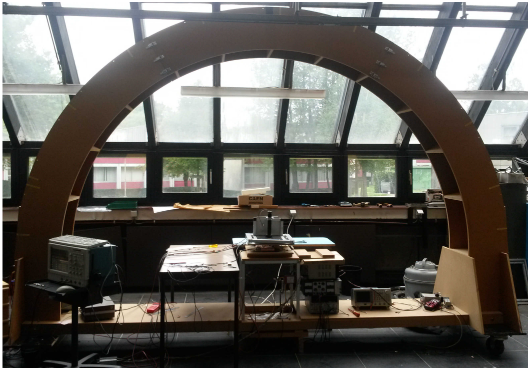
Figure 5.8 – The arch setup with the triple-GEM detector placed between the scintillator sc-bot and sc-top.
