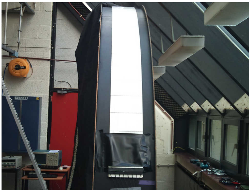
Figure 4.4 – External side of the arch with the scintillator ribbon installed.
