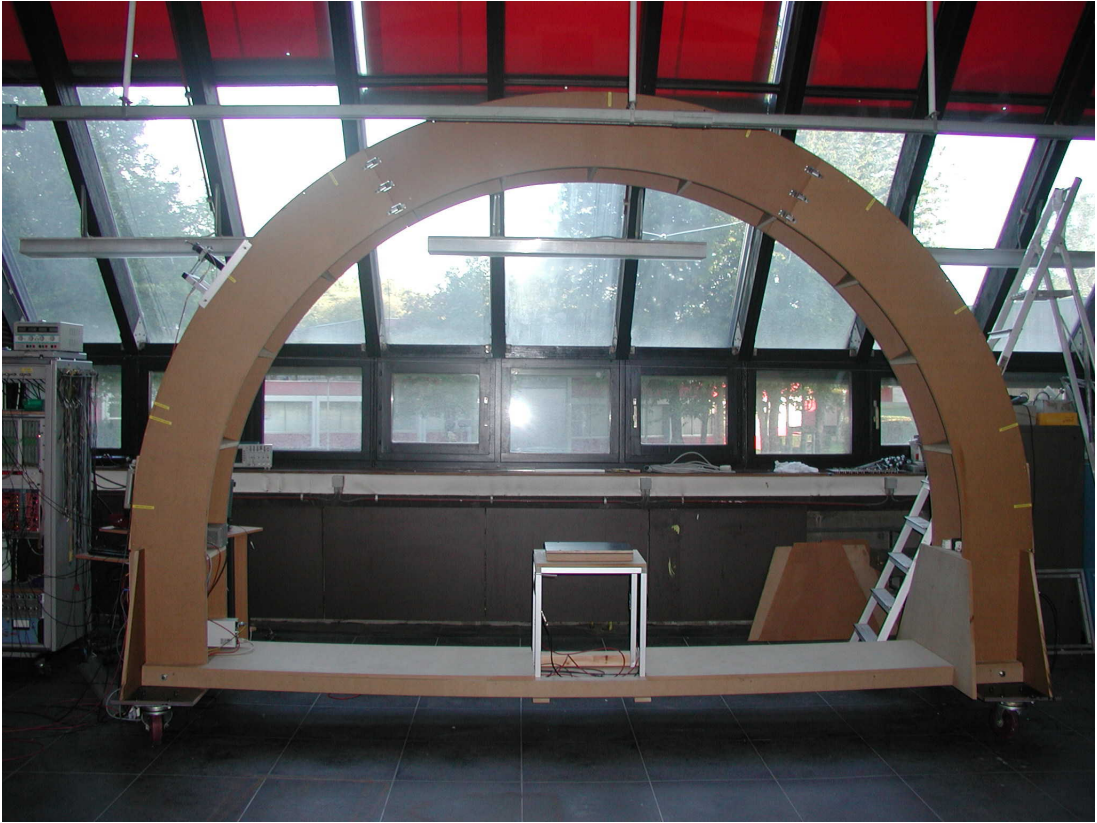
Figure 4.1 – The arch setup with the central table, useful to place other detectors.
