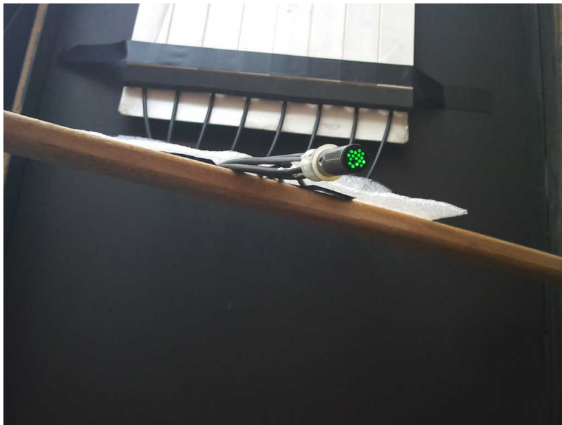
Figure 4.3 – WLS fibers inside the scintillator strips.
