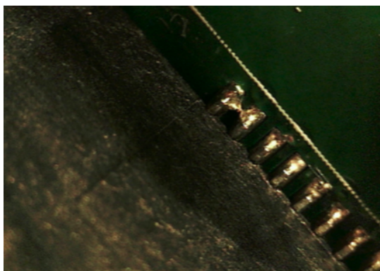
(e) Shorted SAMTEC connector pins (before fix).
