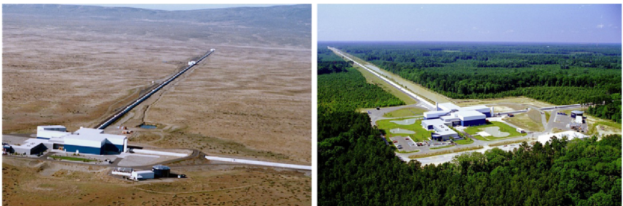
Figure 1.2. Aerial view of the two L-shaped LIGO interferometers: Hanford (left) and Livingston (right). Credit: LIGO Laboratory.
