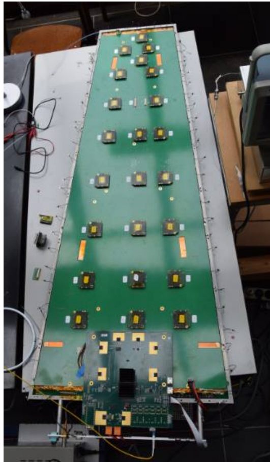
Figure 2.10: Picture of the GEB, the 24 VFATs and the opto-hybrid in the bottom [6].
