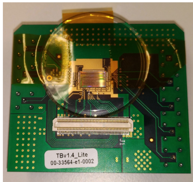
Figure B.5: The translation board v1.4. The VFAT3 chip sits on the bottom side of the board, under a plastic cover to protect the bonding .
