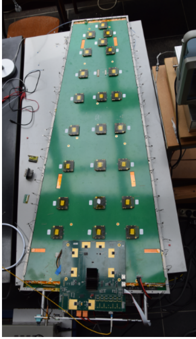
Figure 3.5: Picture of the GEB with the VFATs and the Opto-Hybrid.
