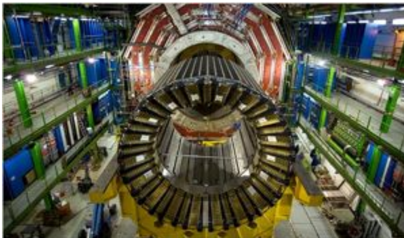
Figure 2.9: Insertion of HCAL in CMS [15]
