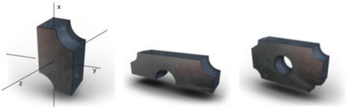
Figure 4.8: Cells able to build up a single GEM, the first one being the primitive cell. [25]
