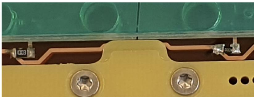
Figure 9.22 – Magnified view of a GE1/1 foil showing a  $10\text{ M}\Omega$  resistor (left) and  $0\ \Omega$  resistor (right) [119]
