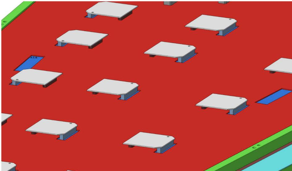
Figure 3.7 – Figure showing the connection of VFAT hybrids (grey) to the GEB. The GEB is shown in red, with holes in the GEB such as those which account for the connectors to the readout board are shown in blue. The external frame of the detector is shown in green. [38]
