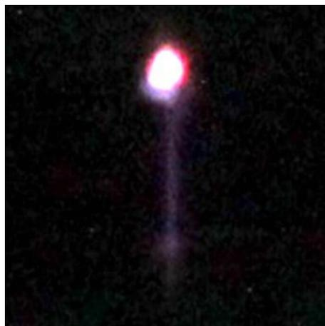
Figure 5.7 – Thermionic emission present in a THGEM with  $E_{ind} = 6.5 \frac{kV}{cm}$  and  $\Delta V_{THGEM} = 1000 \text{ V}$  [91]
