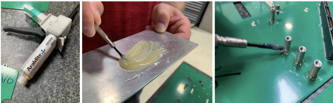
Figure 3.6 – Application of Araldite glue to reinforce the stand-offs on a v3 GEB [41]
