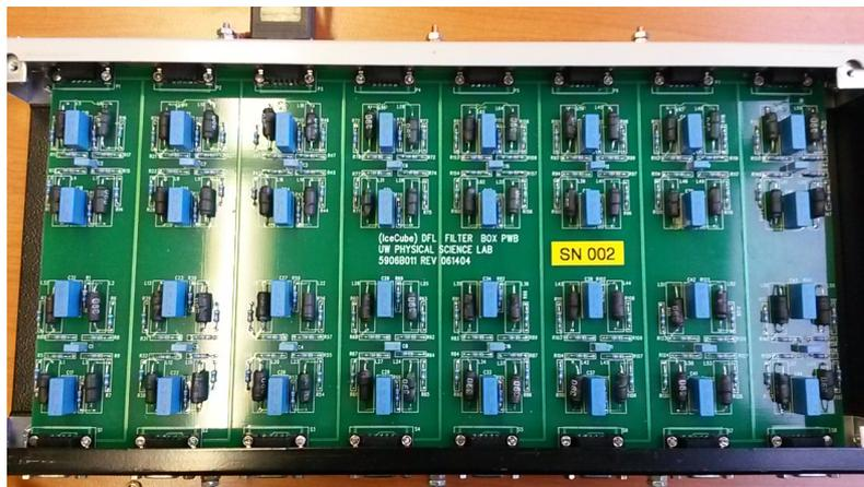
Fig. 10.2.: Inside of a filter box. The same filter schematic is copied in two rows and eight columns, with the passive through hole components clearly visible.
