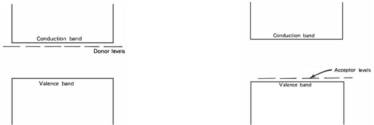
Figure 7.2: Schematic of the modified bandgap structure of an n -doped (a) and p -doped (b) semiconductor. Figures taken from Ref. [173].
