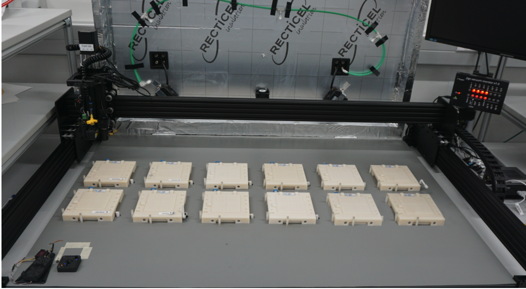
Figure 5.5: A picture of the gluing robot with 12 sensor gluing jigs.
