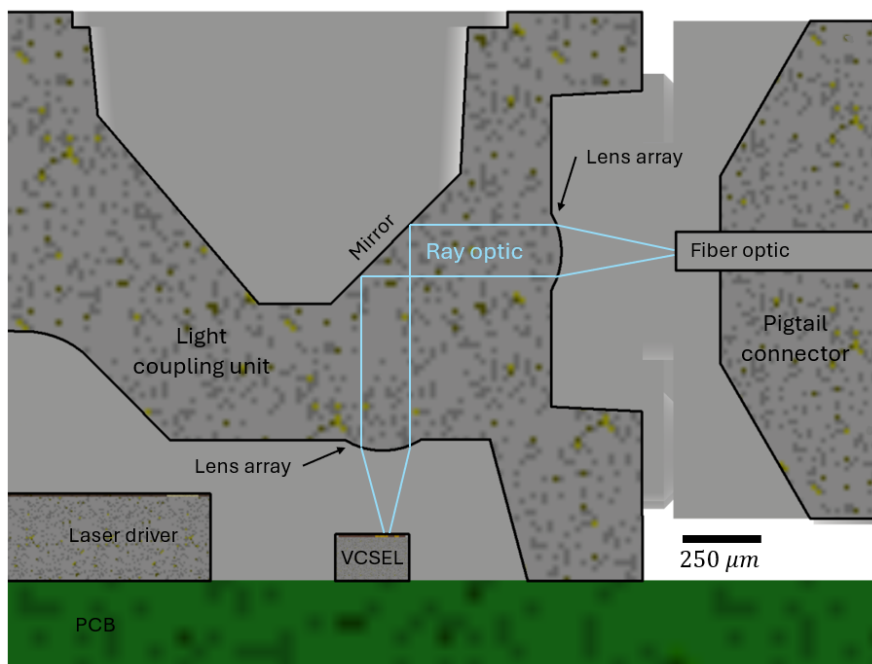
Figure 8.3: Partial 2D cross-sectional schematic of the VTRx+ module, showing selected components including the light coupling unit, VCSEL, pigtail connector, laser driver, and PCB section.
