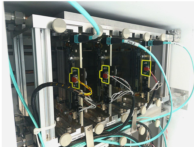
Figure 8.16: Image of the modules on the carrier frame inside the burn-in system. The temperature sensors are highlighted in yellow. The VTRx+ modules are located at the bottom left of the modules in these images.
