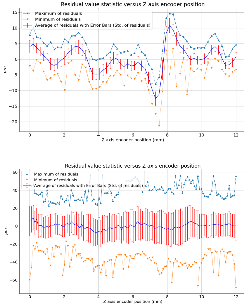
Figure 6.18: Top: The residuals of the measurements on surface of white liquid with the respect to the fitted line. Bottom: The residuals of the measurements on surface of back side of a functional sensor.
