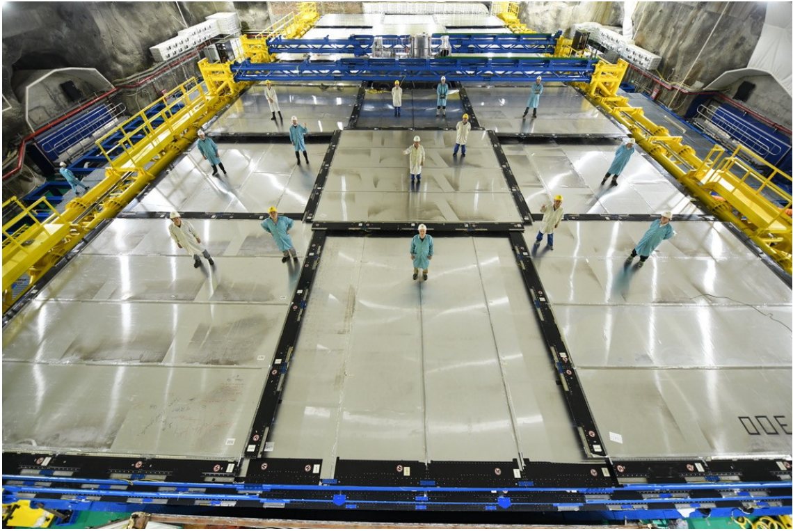
Fig.3 Top tracker above the water pool. (Credit: JUNO Collaboration)
