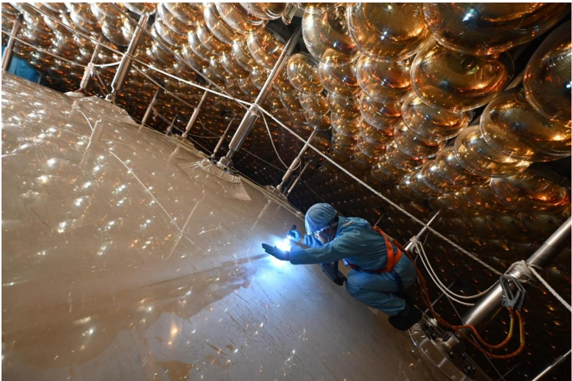
Fig.2 The central acrylic sphere and PMTs. (Credit: JUNO Collaboration)
