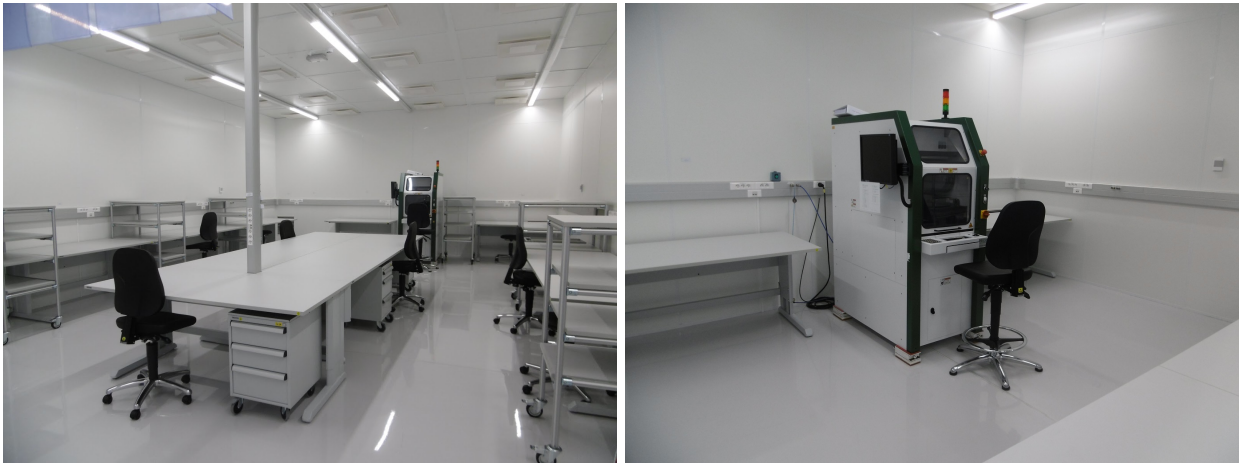
Figure 6: Left: the newly-furnished clean room at the IIHE. Right: the Hesse BondJet820 industrial bonding machine installed at the IIHE.
