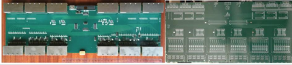
Figure 10: The baseboard of the BEC developed at the ULB (v2 on the left and v3 on the right).
