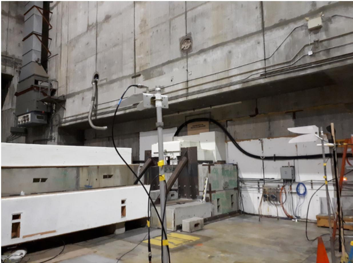
Figure 12: Radio antenna set-up for the SLAC experiment.
