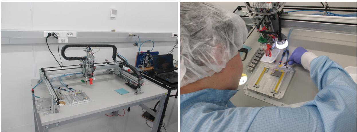
Figure 6: Left: gluing robot developed at the IIHE. Right: first trial assembly using the kapton gluing precision jig.
