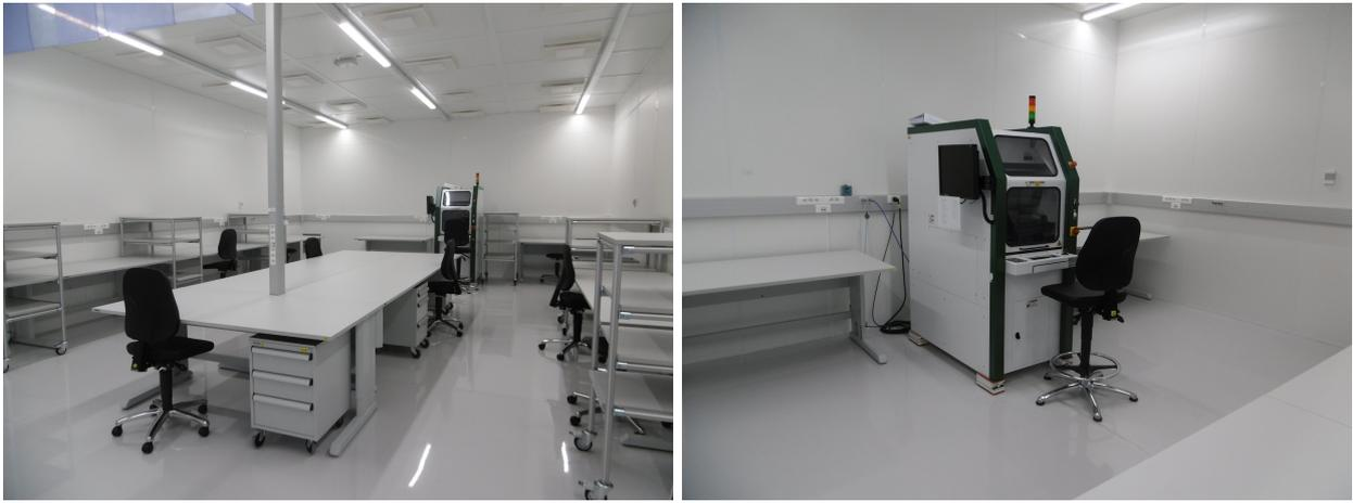
Figure 5: Left: the newly-furnished clean room at the IIHE. Right: the Hesse BondJet820 industrial bonding machine installed at the IIHE.
