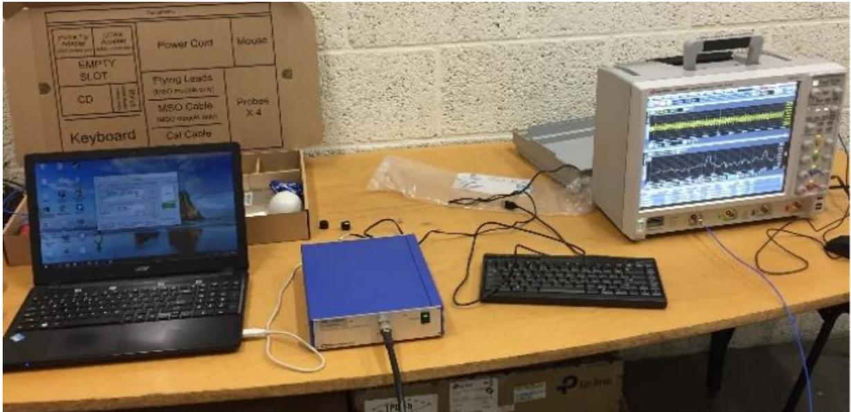
Figure 11: Construction of the DAQ for the calibration set-up at the IIHE. The radio detection set-up used at the SLAC experiment are calibrated.
